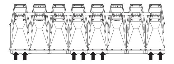
**Step 2.** Using the bolts supplied with the speaker, tighten the suspension brackets and side angle plates. Combine the brackets supplied with the two speakers, and attach them with the suspension holes facing outward, as shown in the figure below.
