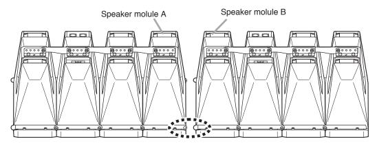
Join the side angle plates using the supplied bolts, spacers and rubber rings.
