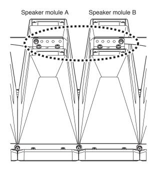
**3-1.** Attach the HY-CN7 bracket's rear angle bar to the rear bracket of speaker module A. Use the supplied hex head bolts and nuts.
